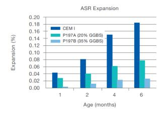
The presence of GGBS effectively reduces the concrete permeability and the Alkali content in the cement. Hence, the chemical resistance of concrete is improved. With GGBS content up to 35% P197A and P197B provide moderate resistance against chloride penetration, sulphate attack and Alkali-Silica Reaction (ASR). For concrete under aggressive chemical environments, higher GGBS content is required.
