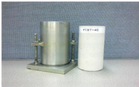
A 7-day cured P197-4S sample with a \phi 50 \times 100 mm cylinder mould for compressive strength test
