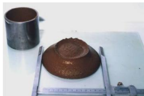
The flowability of sludge and/or stabilizer is measured using a flow ring with a dimension of \phi 77
