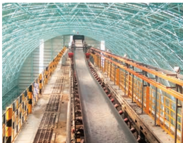
Photo: Slag transport to vertical roller mill by conveyor belt
