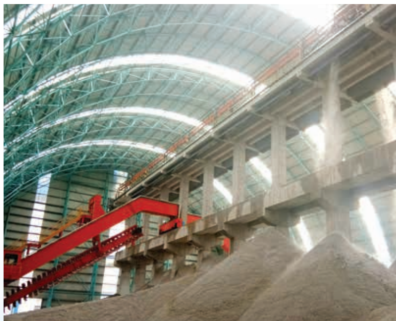
Photo: Slag receiving and storage in an enclosed system
