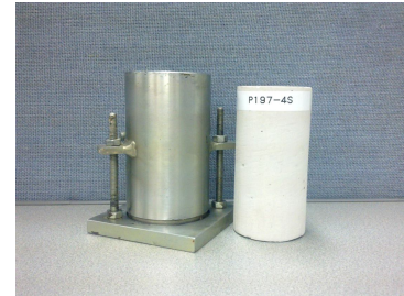
A 7-day cured P197-4S sample with a \phi 50 \times 100 mm cylinder mould for compressive strength test.
