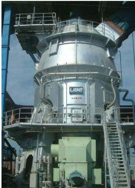
UBE Vertical Mill UM46.4SN (Made in Japan) is employed at TL JV's 2 nd production line
