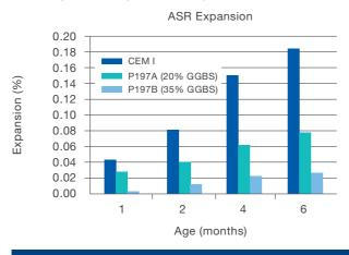
The presence of GGBS effectively reduces the concrete permeability and the Alkali content in the cement. Hence, the chemical resistance of concrete is improved. With GGBS content up to 35 %, P197A and P197B provide moderate resistance against chloride penetration, sulphate attack and Alkali-Silica Reaction (ASR). For concrete under aggressive chemical environments, higher GGBS content is required.
